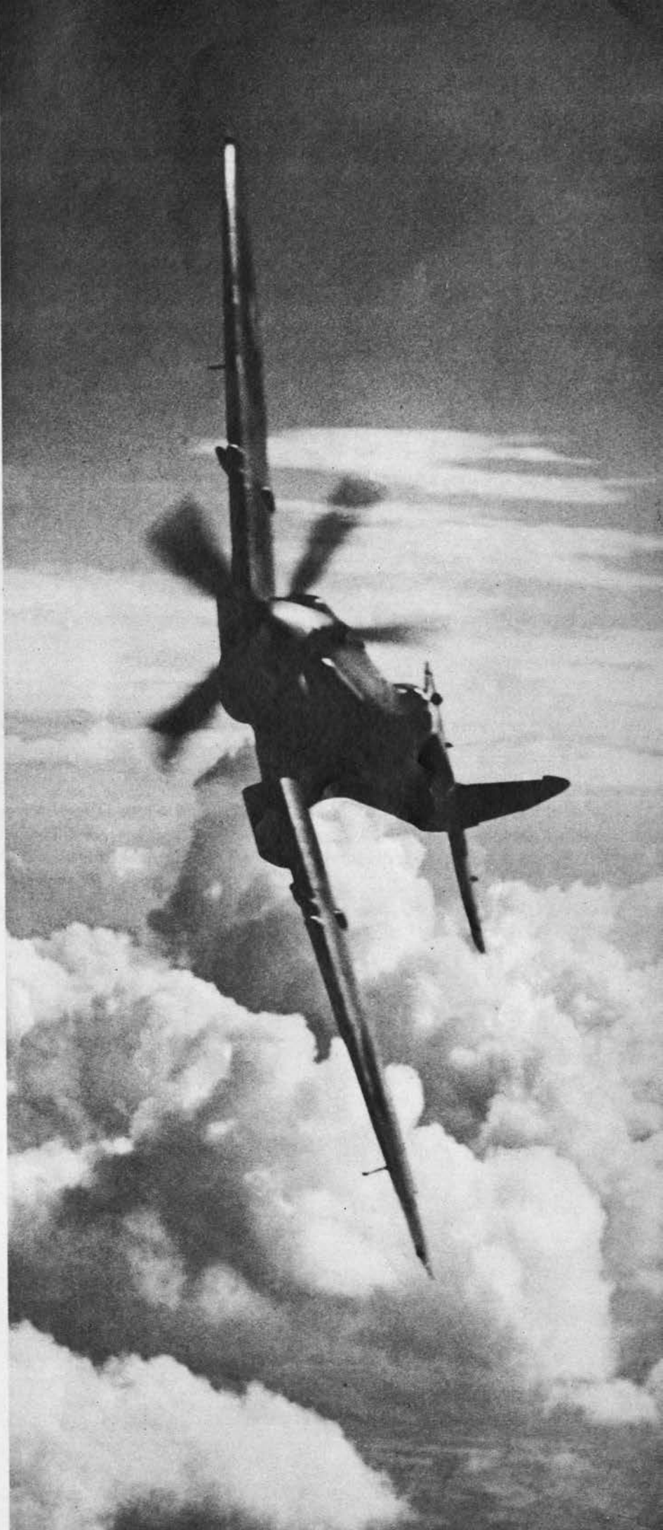
SPITFIRE XIV Frequently modified, the Spitfire is still among world's best. Broader fin and rudder, deeper radiators and a longer nose distinguish it from the Spitfire IX.
